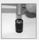
STEP 6 Place the TOOL (20) over the rear portion of the REFLECTOR (5).
