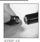
Before installing the batteries, check for leakage or corrosion. Reinstall or replace the batteries, (one/AAA series alkaline only) install with the positive (+) end toward the lamp. Reinstall TAIL CAP (14).
