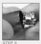
Replace the REFLECTOR (5). Place the REFLECTOR (5) into the opening of the HEAD (2) being careful not to get fingerprints on the reflective surface.
