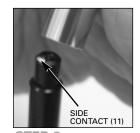
Insert the TOOL (20) with the LOWER INSULATOR (13) into the bottom of the BARREL (10). Push the TOOL (20) into the BARREL (10) until it stops at the top of the BARREL (10).
